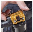
Alternatively tightening of each bolt in a cross pattern in small turning degrees helps to evenly distribute the pressure applied by each bolt into the stem cap and the handlebar. This improves the grip of the stem cap and avoid damages to the handlebar.
