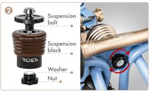
Insert the suspension bolt through the block. Place these parts in the frame. Screw the nut into the suspension bolt (do not forget to place the washer first) and tighten it. To tighten the nut, you can use a 19 mm spanner.
