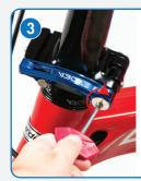
Install the original cap and tighten the bolt with a T20 wrench. Using mild threadlocker is recommended.
