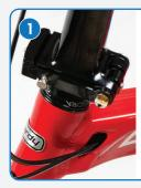
Remove the original hinge clamp. Keep the following original parts: spacer, cap, bolt.
