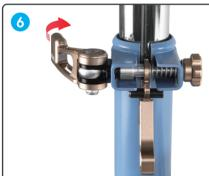
With the QR in the open position, tighten the nut manually until a position where the QR lever leaves you a slight pressure mark in the palm of your hand after closing it.
