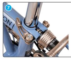
Secure the rear wheel and make sure that the frame release holds it in position. You can lift the bike and shake it, or drop it to the ground, to test that the bike is safe to ride. Release the rear wheel and secure it several times before riding for the first time.
