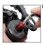
2 Use the supplied special extractor tool and a 5 mm hex wrench to remove the body screw. Caution: please press the pulley cage against the derailleur to avoid an abrupt release of the spring tension.
