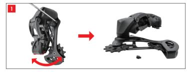
Rotate the pulley cage forward and press the cage lock button to lock the derailleur. Remove the pulley cage stop screw using the 3mm hex wrench. Release the cage lock and carefully allow the pulley cage to unwind. This will release the tension from the spring. Your derailleur should appear as in the photo of the next bullet.
