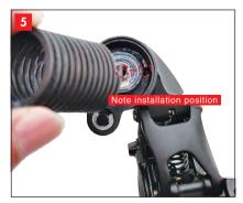
Be sure that the tip of the spring remains in the installation hole of the body. Place it properly if it moved when you removed the pulley cage.
