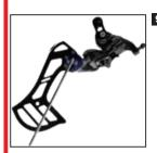
9 Fix and take the screw about 3 turns first. Let the limit screw to rotate and pass through the stopper's upper flat.
