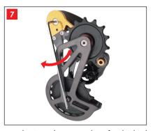
Use the 3mm hex wrench to fix the body to the OSPW evo. Tight to 4 N.m.
