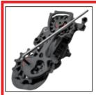
2 Disassemble the original rear derailleur cage and pulleys. PS. 3mm hex wrench
