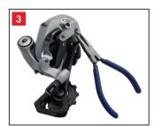
Use the needle nose pliers to take out the tenon after rotating.
