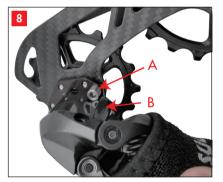
Please fix and rotate the limit screw in front of the stopper, and hold the derailleur body and plate tightly.
