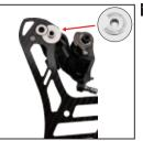
12 The side cap's gap of upper pulley must to be aimed at fixing bolt.
