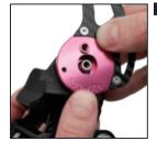
Apply some grease onto the cage-body interface of the OSPW<sup>†</sup> outer plate. Align it with the spring so the hook fits in the spring tension hole of the plate.
