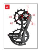
2S is the Standard tension setting and the one we recommend to start with. Then, in case you need lower tension and friction on the chain you can switch to 1L, which is the Low tension setting, to see if that works better for you. On the contrary, in case you want better shifting performance, you can switch to 3H, which is the High tension setting, to see if the increased tension and friction of the chain works for you. PS. U1 U2 is suitable for old models SHIMANO springs.
