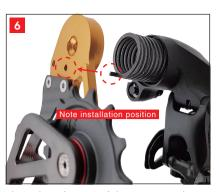
Place the other tip of the spring in the tension hole of the OSPW evo and compress the spring to close the gap.
